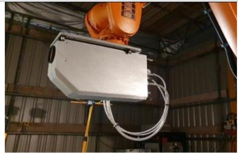
**Figure 4** Optical laser head on the end effector of the KUKA robot arm
